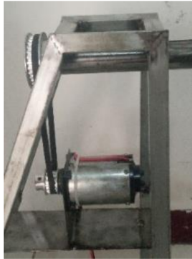
Figure 8. Coupling between a wind turbine and generator (Source: Personal data)
