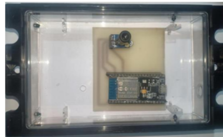
Gambar 25. Alat Monitoring Suhu Klem 20 kV
