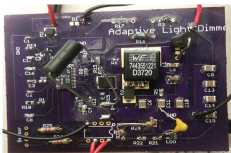
Figure 9. Adaptive light dimmer hardware prototype
