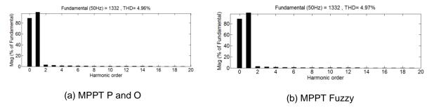
Figure 12. Current harmonics spectra of phase A under 1Ph-N fault
