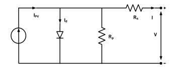
Figure 3. Equivalent circuit of solar panel
