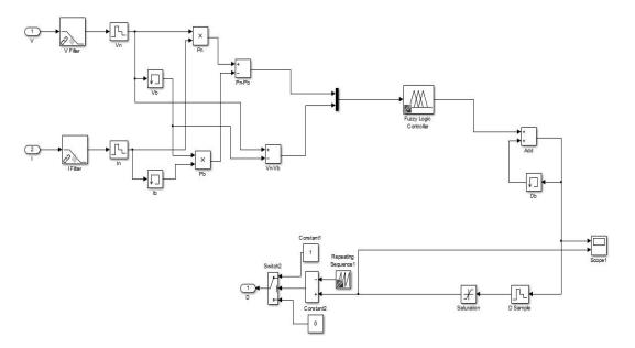
Figure 7. Matlab/Simulink for MPPT Fuzzy
