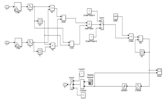
Figure 5. Matlab/Simulink for MPPT P and O
