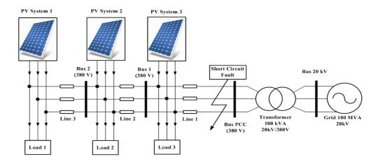
Figure 2. Proposed model of multi PV connected three phase grid under short circuit fault
