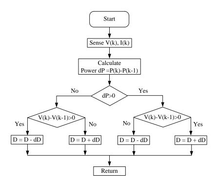
Figure 4. MPPT using P and O algorithm
