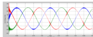
Figure 10 Phase voltage of three phase four wire distribution network on PCC bus before multi units of single phase PV DGs combined with BES
