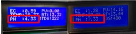
Figure 14. Performance measurement of pH-Up at 08.00 and 14.00 hours
