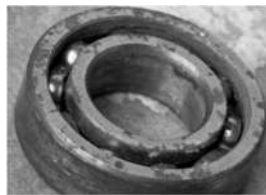
Figure 2. A Bearing fault caused by corrosion
