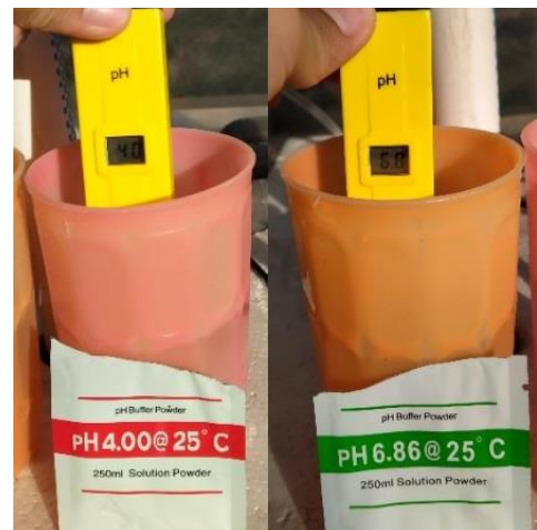
Figure 12. pH measurement using digital-meter
