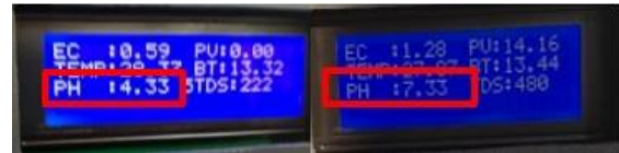
Figure 15. Performance measurement of pH-Up at 08.00 and 14.00 hours
