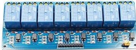
Gambar 2.9 Module Relay Channel. [7]
