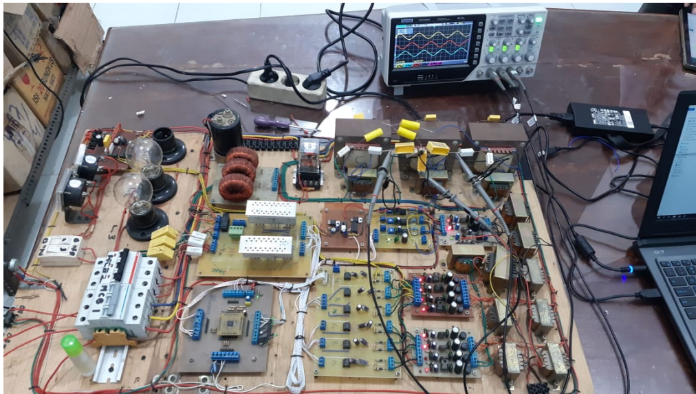
Fig. 5. Design and implementation of AC-AC converters on a laboratory scale.
