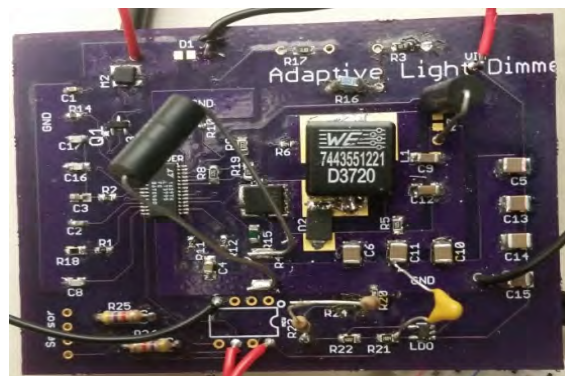
Figure 9. Adaptive light dimmer hardware prototype
