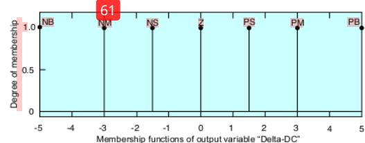
Figure. 9 Output MFs of MPPT-FS ( $\Delta D$ )
