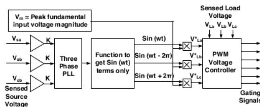
Figure. 4 UVTG control of series active filter
