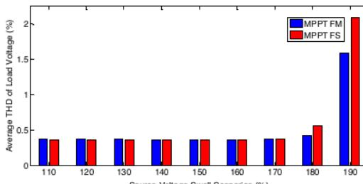
Figure. 19 Performance of average THD load voltage for voltage swell
