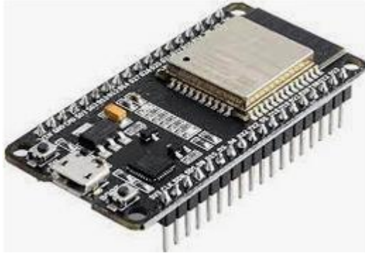
Gambar 2.8 Modul ESP32 devkit-C
