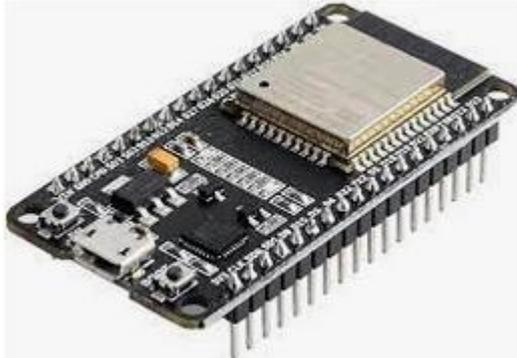
**Gambar 2.4** Modul ESP32 devkit-C
