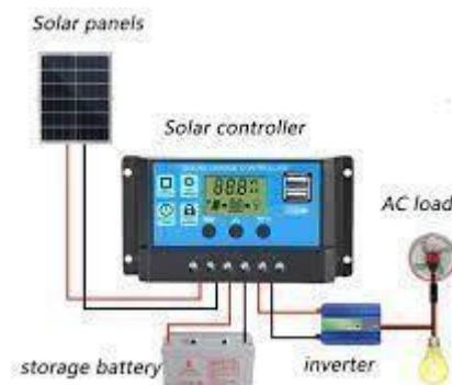
Gambar 2.4. Solar Charge Controller
