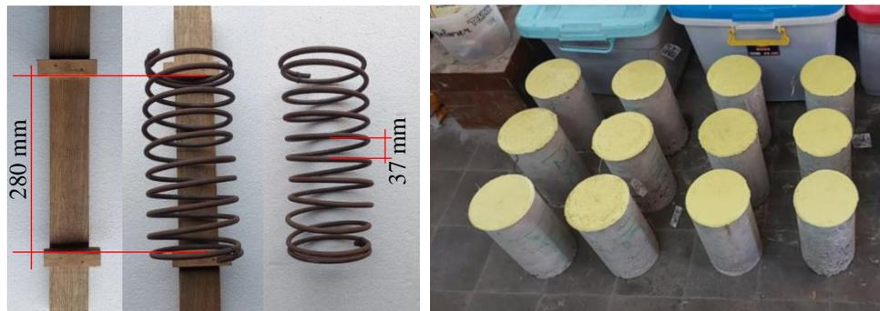
**Figure 3** Details of spiral with  $\phi = 8$  and  $S_h = 37$  mm (the specimens had no longitudinal or main steel bars) and ready-to-test capped concrete specimens
