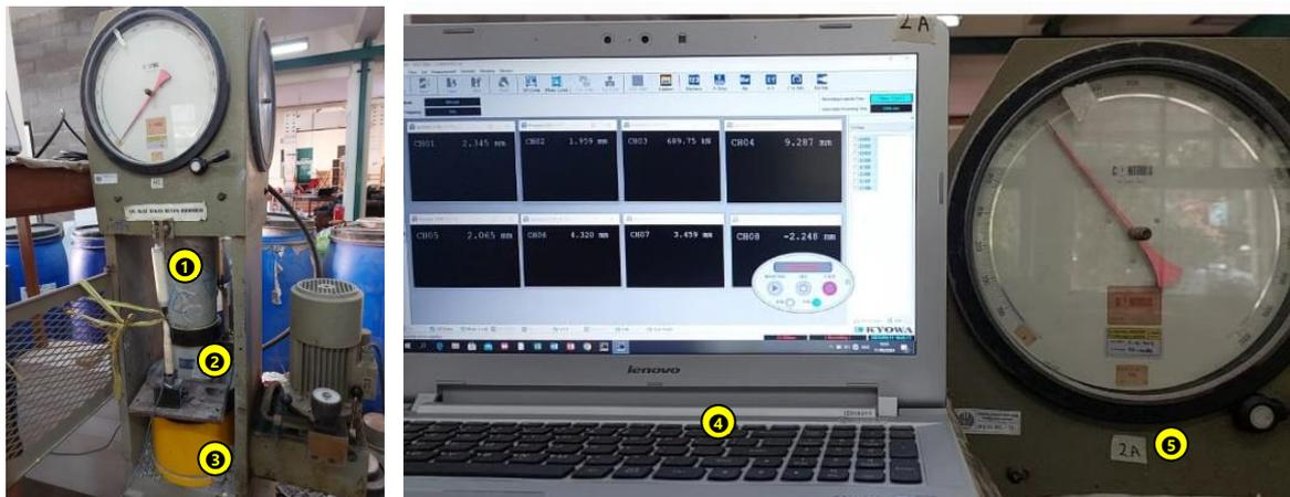
**Figure 4** Actual test setup: ① LVDT (Linear Variable Displacement Transducer) vertical, cap. 50 mm; ② single-acting load cell, cap. 1 MN; ③ single-acting hydraulic jack, cap. 200 kN; ④ computer; ⑤ manometer
