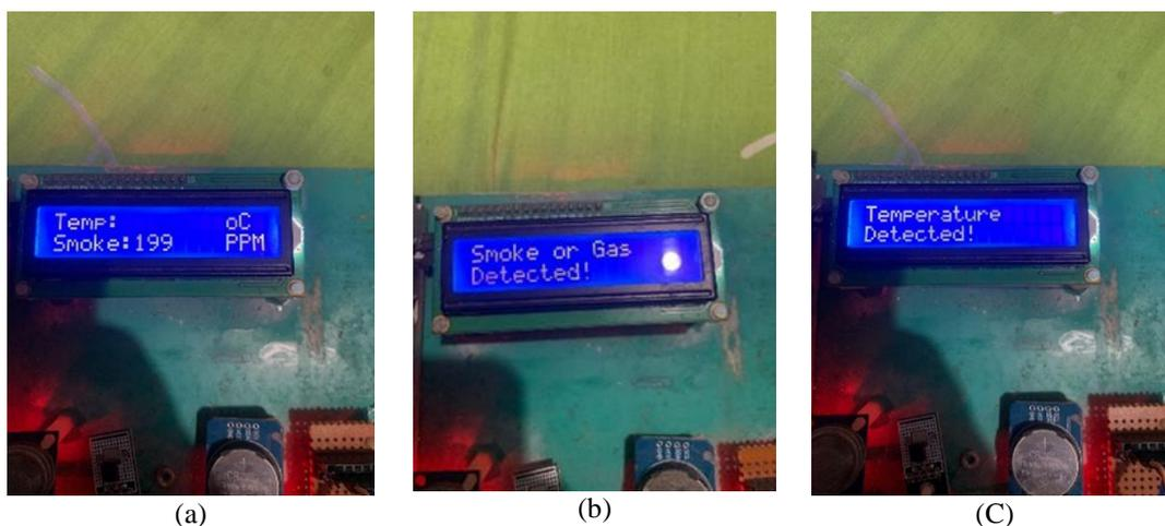
Figure 10. LCD screen display in tool mode conditions: (a) Standby, (b) Detecting smoke (gas), and (c) Detecting temperature
