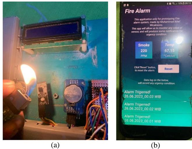
Figure 8 (a) Match temperature test using the LM35 sensor, (b) Results of testing temperature values at three different match source distance positions
