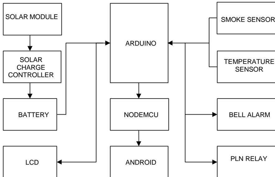
Figure 1. Prototype Design of Fire Early Warning System in Residential Houses
