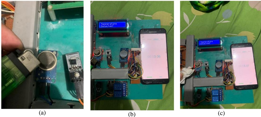
Figure 7. (a) Testing using the MQ-2 Sensor, (b) Results of testing the sensor on lighter gas, (c) Results of testing the sensor on cigarette smoke
