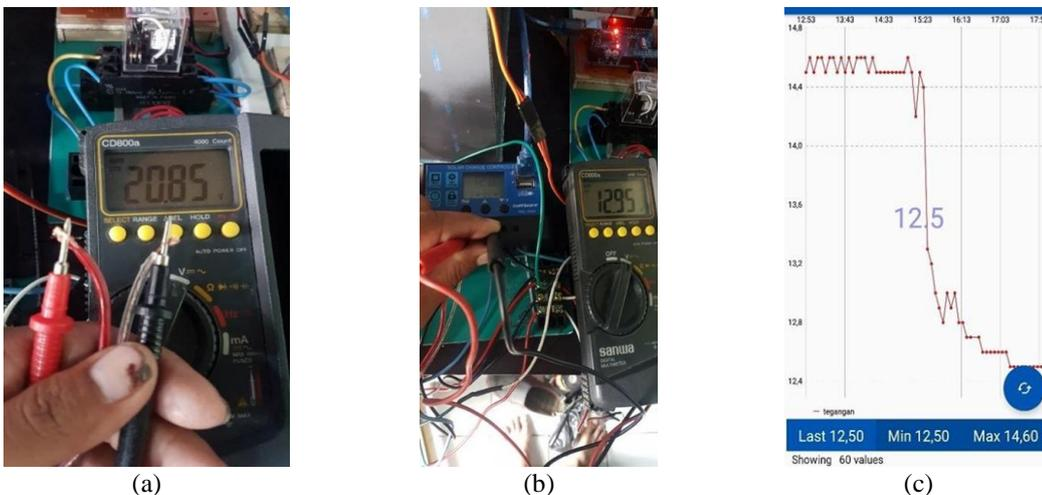
Figure 5. (a) Measurement of solar module output voltage, b) Measurement of battery output voltage, c) Graph of battery output voltage measurement results
