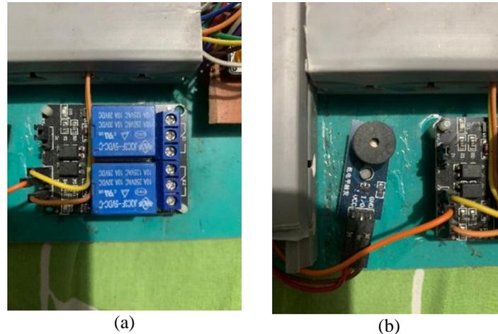
Figure 9. Test of the working mechanism of (a) the breaker relay and (b) the buzzer
