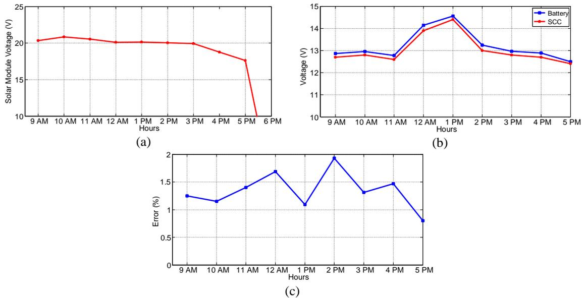
Figure 6. (a) Output Voltage of Solar Modules, b) Comparison of Battery Output Voltage and Solar Charge Controller Voltage, (c) Error Measurement between Battery Output and Solar Charge Controller Voltage
