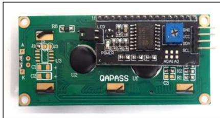
**Gambar 2.11** Liquid Crystal Display 2x16 Tampak Belakang<sup>[45]</sup>
