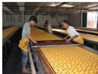
Figure 4. process of printed batik (Sumber: batikpekalongannahdia.blogspot.com/2017/05/jenis-jenis-batik.html)
